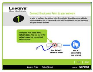
Figure 5-2: Connect the Network Cable to the Router or Switch Screen
